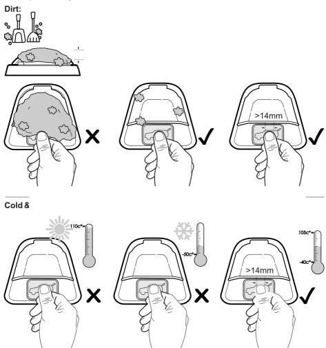
**Immunity**: The Capacitive Touch Pad has been configured to ignore un-intended triggers when exposed to the following conditions: Carwash, Direct Hose, Dripping Water, Wind, Dust, etc. however the immunity of the Touch Pad cannot be guaranteed in all user cases.
