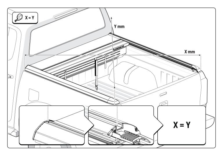
• Ensure the cross measurements are identical.
