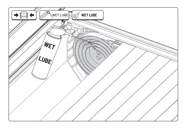
Regularly, and following cleaning, apply a PTFE-free all-conditions wet lube product to the inside of the canister ends.
