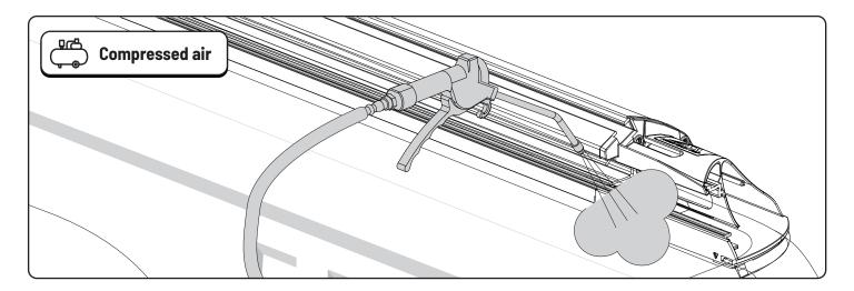
Remove dirt and debris using compressed air.
