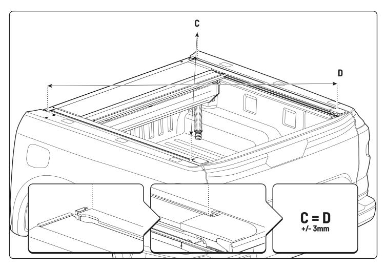
• Ensure the cross measurements are identical.
