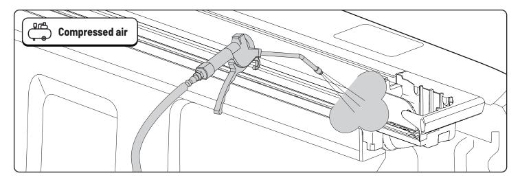
• Remove dirt and debris using compressed air.
