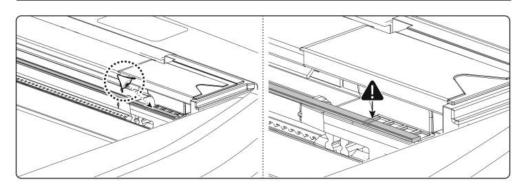
• If abnormal sounds occur during operation of the roll cover, inspect the glide rails for debris or damage. If the glide rails are damaged or worn, then replacement glide rails are needed.
