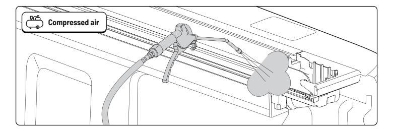
Remove dirt and debris using compressed air.
