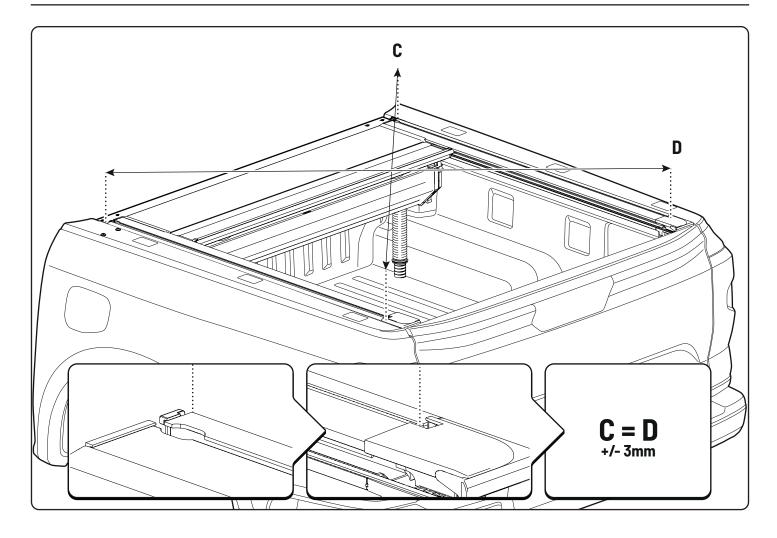
• Ensure the cross measurements are identical.
